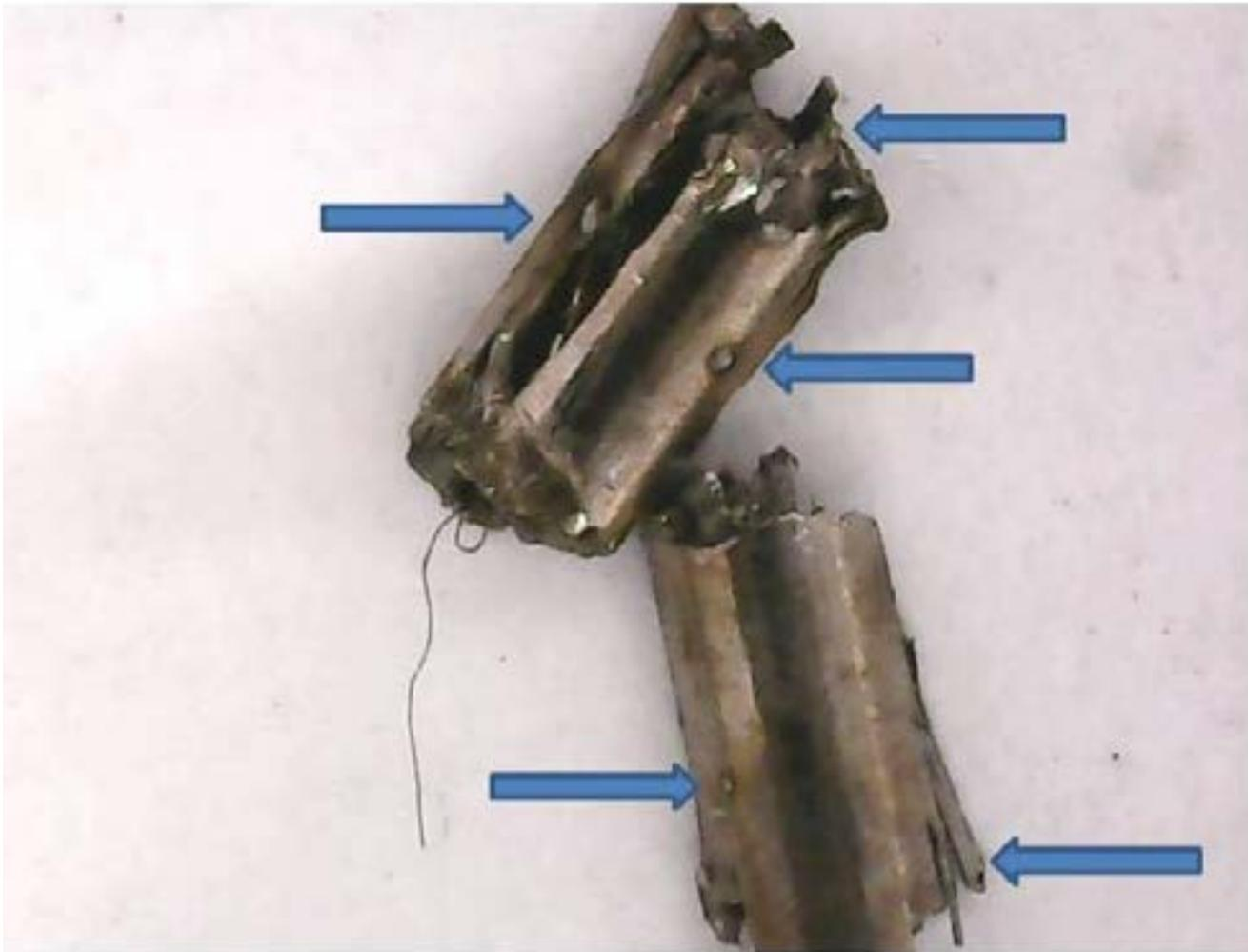
**Tungsten cylinders with craters and cracks**
