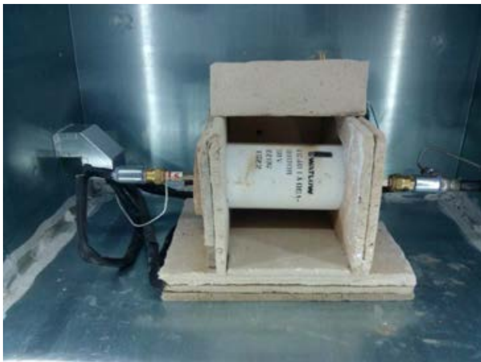
Fig.5 Reaction tube in the heater, in the safety box
