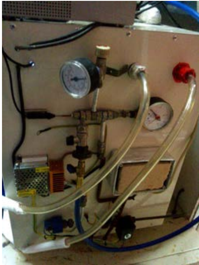
Fig.13 Reactor pressure control
