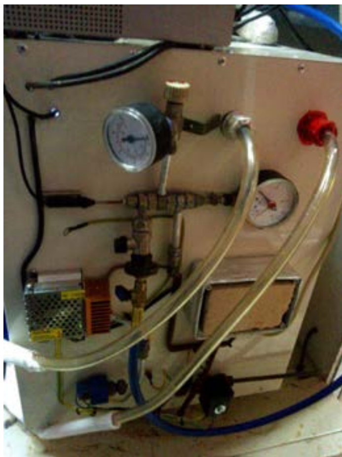
Fig.13 Reactor pressure control
