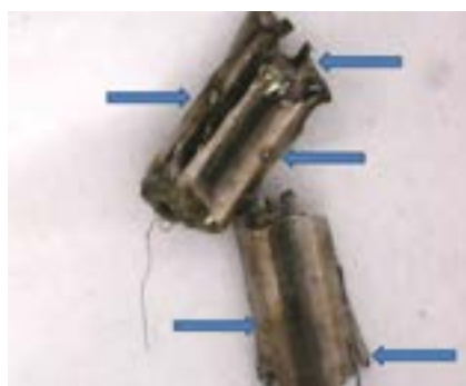
Tungsten cylinders after reaction, with craters and cracks
