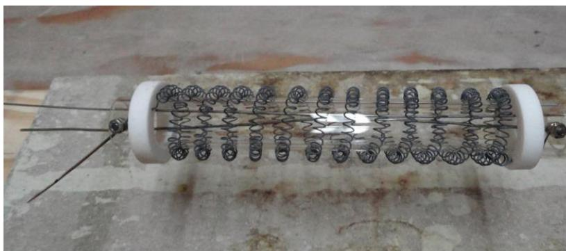
Figure 1: Oxidized Ni Wire Wound Around Quartz Tube
