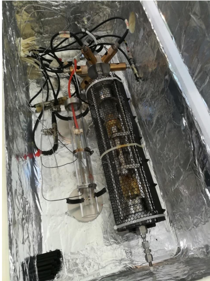
Fig. 9_M. Picture of the reactor, and calibrator (Ni-Cr wire) inside the calorimeter (advanced version, comprising 2 insulating and reflecting walls)
