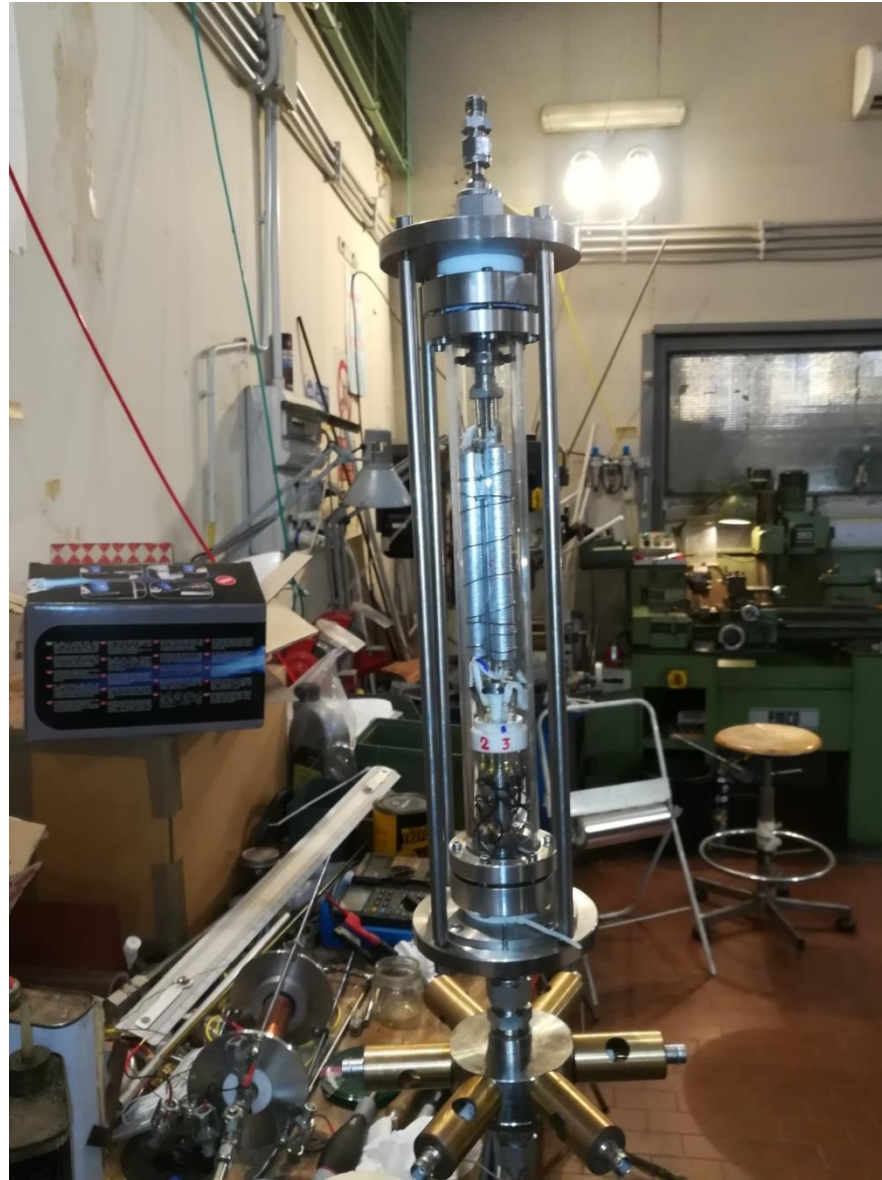
Fig. 8_M. Photo of the reactor assembled, just before to be located into the air flow calorimeter.
