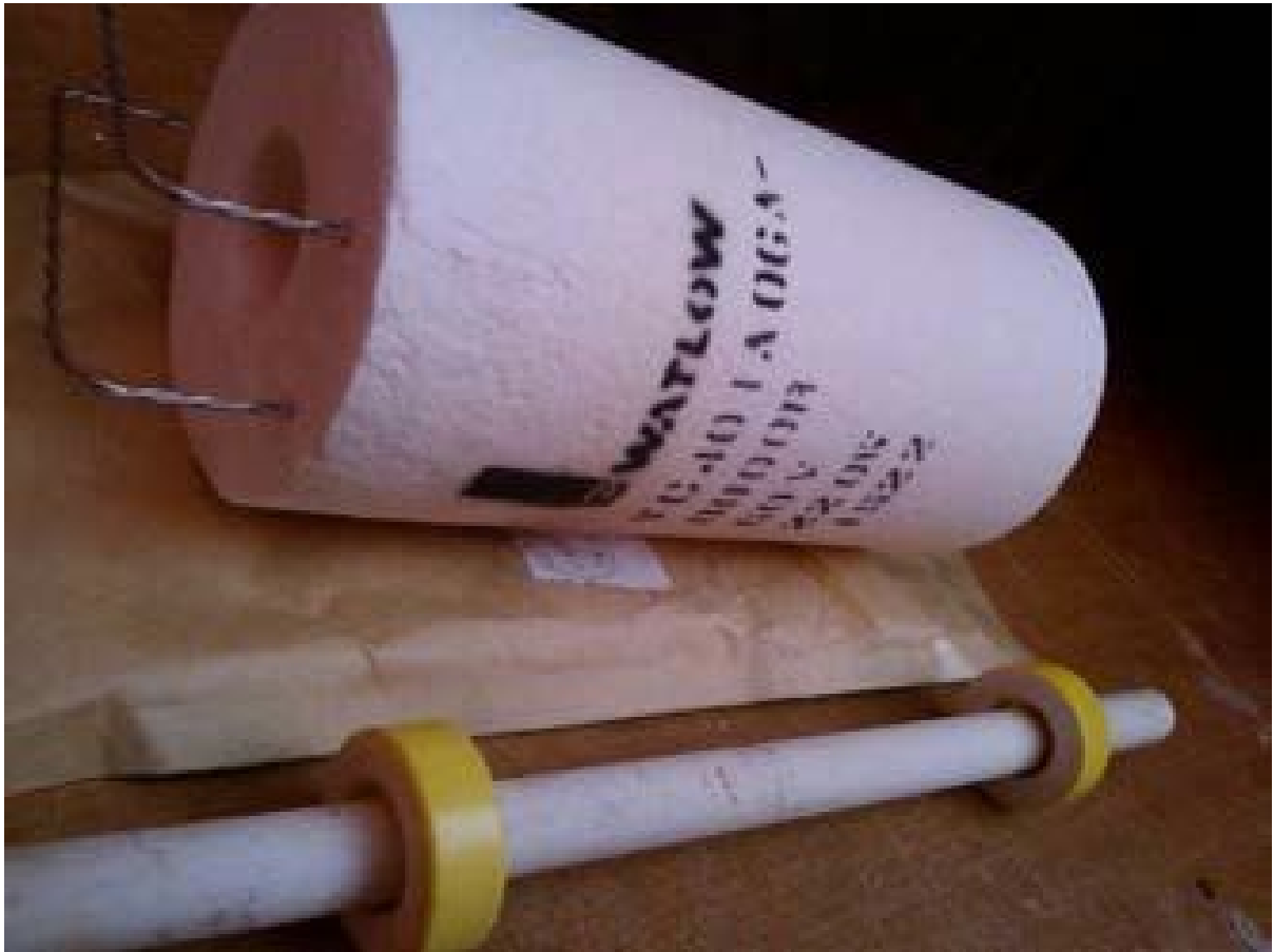
Inserting the reactor tube spacer locks
