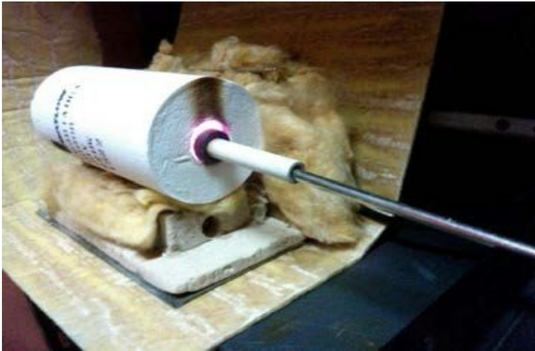
Watlow heater in operation test
