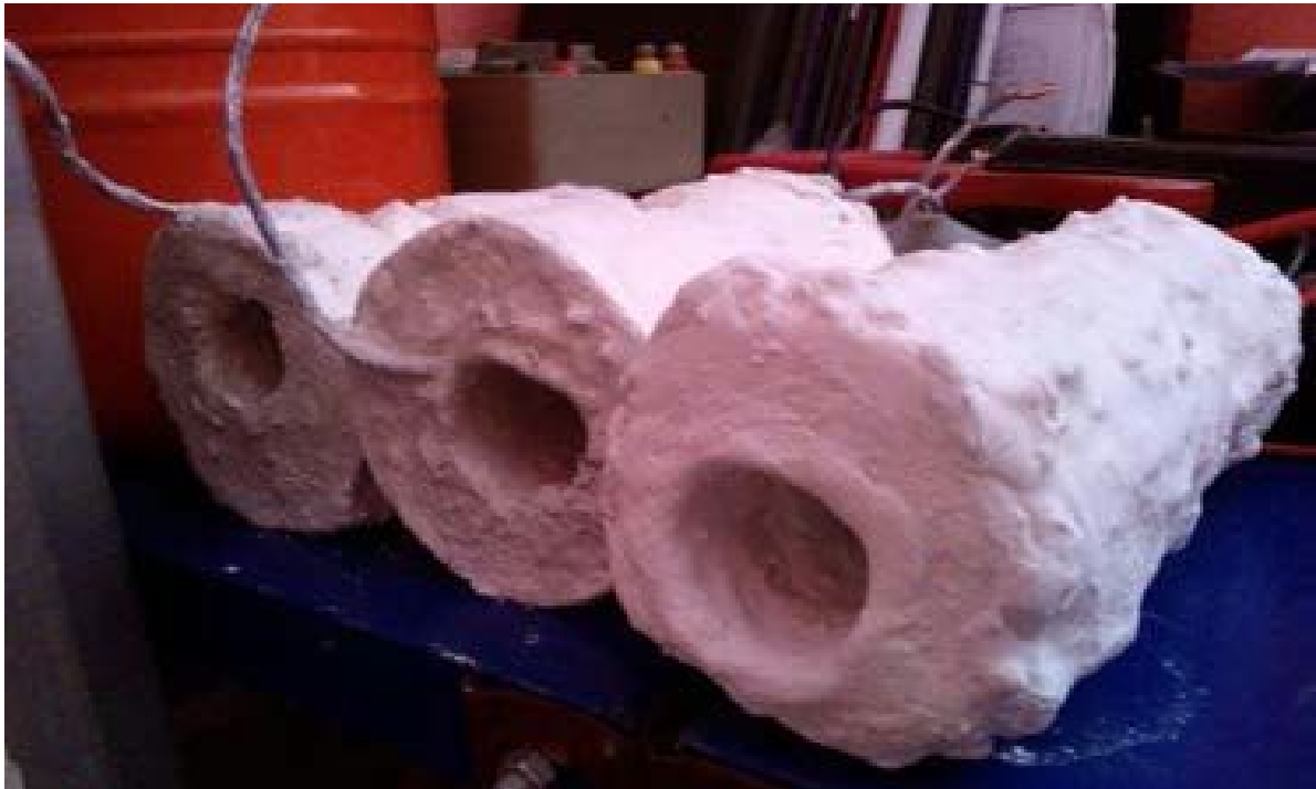
Copies of the Watlow heater, ready for finishing
